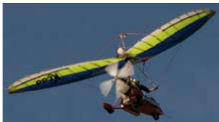
The FZK-ENDURO (DE) is the smallest aircraft of the fleet, with a scientific payload of 80kg and an endurance of 5 hours at a sampling speed of 25 m/s.
